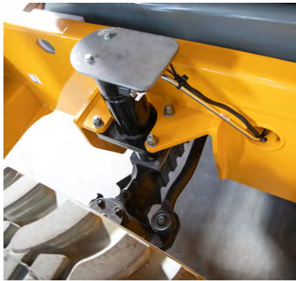
Mechanical axle drive design uses fewer hydraulics
