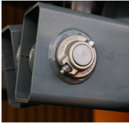
Anti-corrosion treatment on axles, fasteners and painted components
