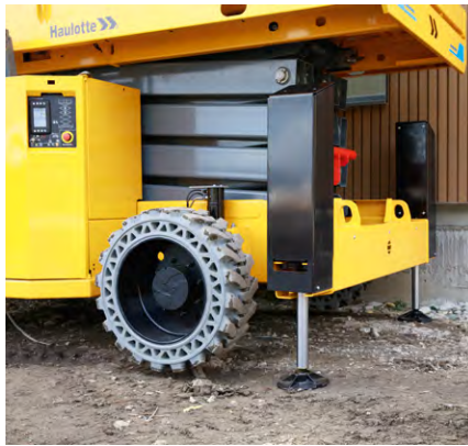
Reinforced covers to protect the outriggers
