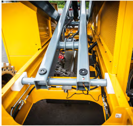
Carefully designed guide for wires and hoses
